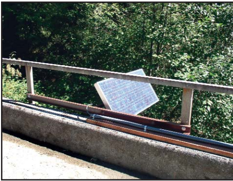
The system's solar panel was mounted off the side of a bridge spanning the Cedar River to avoid shading from the surrounding forest.
